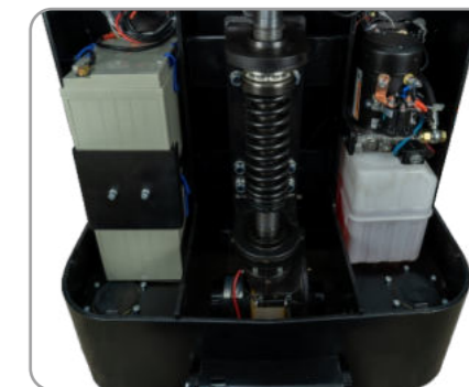
Interior structure Maintnence battery Floating mechanism Built-in charger
